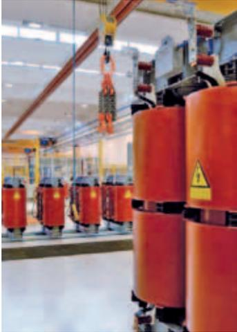
Cast resin transformers production plant
