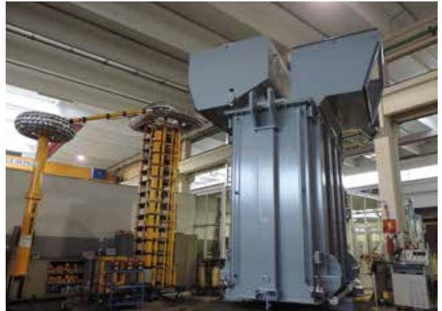
**THREE-PHASE LIQUID IMMERSED CONVERTER UNIT MADE BY TWO TRANSFORMERS IN ONE TANK**
